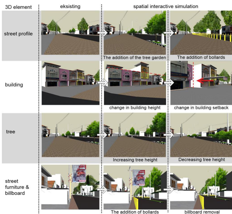
Figure 7. An example of the test running simulation of the spatial multimedia system
