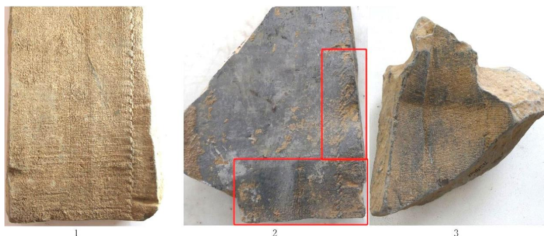
Figure 57 The fabric impressions on the concave surface of the roof tiles
