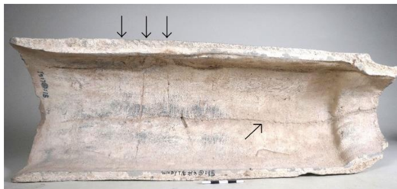
Figure 14 Joint line of clay-strips and traces of the cloth cover's seam on the concave surface of an imbrex (Source: Photo by the author)
