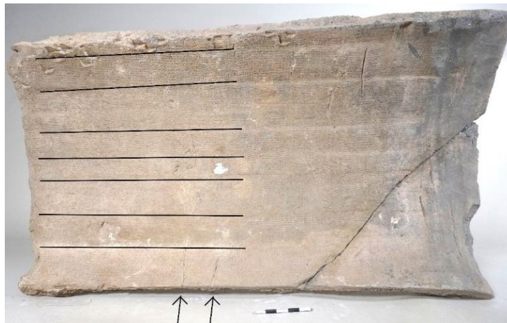
Figure 13 Vertical impression of the wooden strips and joint line of clay-strips on the concave surface of a tegula (Source: Photo by the author)
