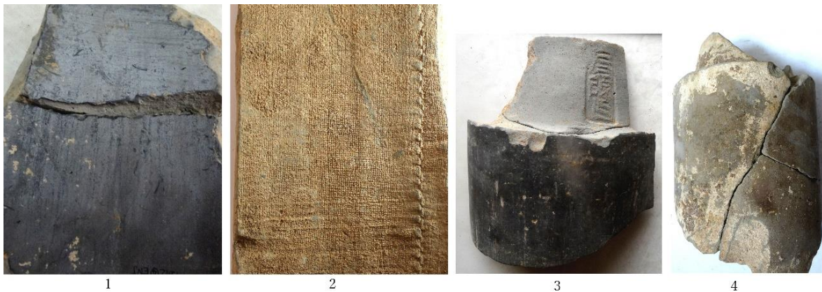
Figure 51 The exposed surface of the roof tiles (Source: Photos by the author) 1. Polished-black tegula, 2. Untrimmed tegula, 3. Polished-black imbrex, 4. Simply-trimmed imbrex
