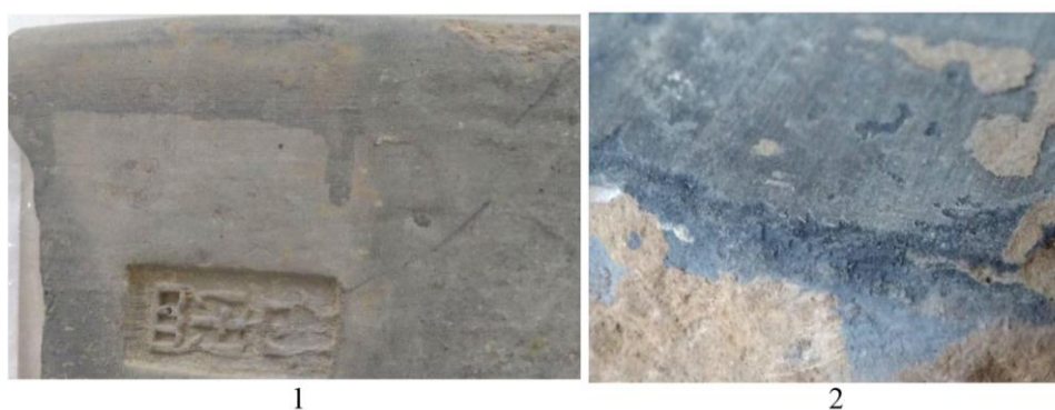
Figure 65 The black liquid and polishing traces on the surface of the tegulae (Source: Photos by the author) 1. Traces of black liquid; 2. Polishing traces
