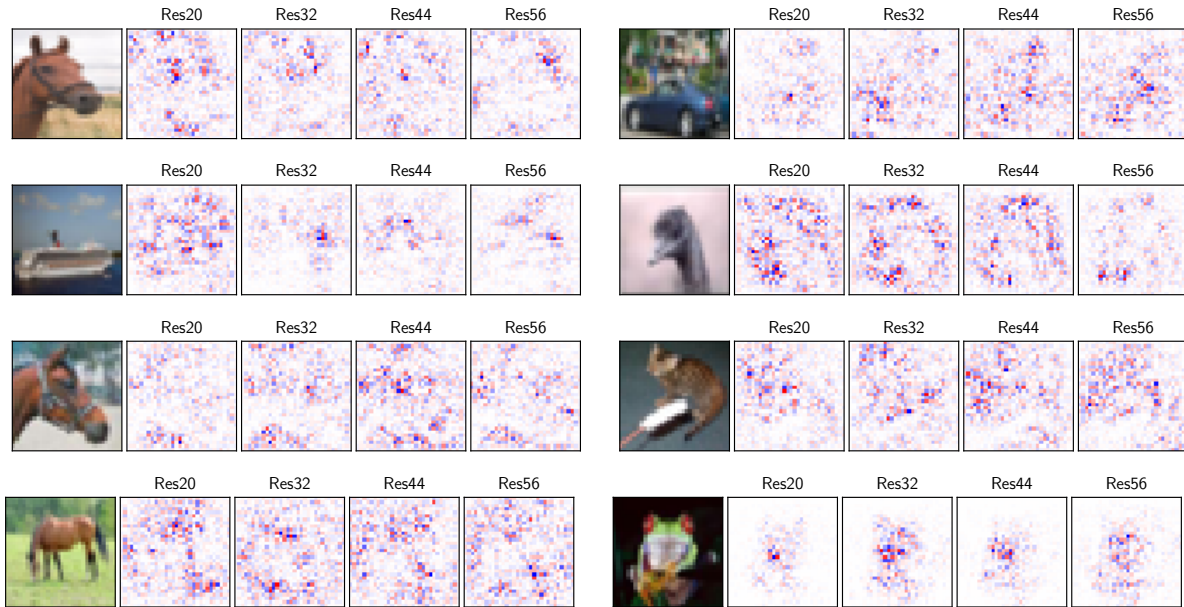
Figure A7: ‘Input×Gradient’ evaluated on different ResNets. Since ResNets are piece-wise linear functions, s.t. y(\mathbf{x}) = \mathbf{M}(\mathbf{x})\mathbf{x} + \mathbf{b}(\mathbf{x}) , this is the ResNet-based equivalent to the CoDA-Net contribution maps.
