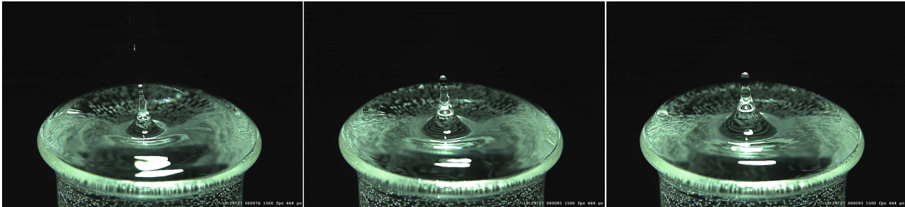
Figure 3 Surface tension behavior of water or simply falling water drops on water surface recorded by 1500 fps. Between the first (Frame 76) and the second picture (Frame 85) are 5976 \mu\text{s} and between the second and the last picture (Frame 93) are 5312 \mu\text{s} . (© D. Curticapean - Offenburg University)
