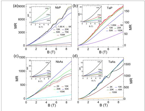
**Figure 1.** Estimated transverse magnetoresistance at different temperatures from the field dependent resistivity using  $MR = \rho_{xx}(B) - \rho_{xx}(0)/\rho_{xx}(0)$  for (a) NbP, (b) TaP, (c) NbAs, (d) TaAs. Inset show their respective magnetoresistance at high temperature  $\geqslant 150$  K.
