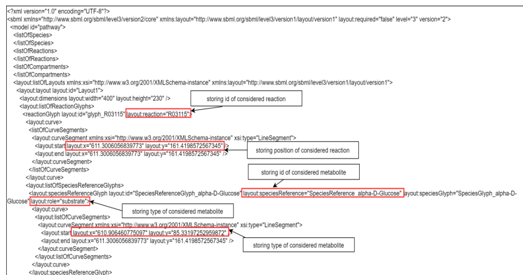
Figure 6. An example of updates in an SBML file. In the tag 'layout:listOfLayouts', all positions for the nodes of the created pathway are stored.
