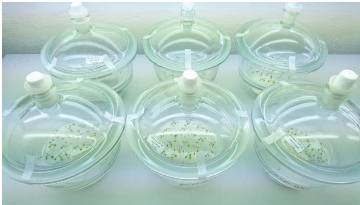
Figure S2. Experimental set-up for fungi- Arabidopsis co-cultivation in a desiccator with shared headspace.
