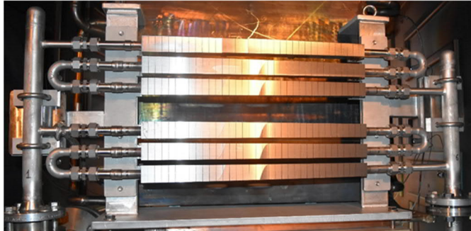
Figure 10: Assembly of 6 PFUs for HADES high heat flux testing
