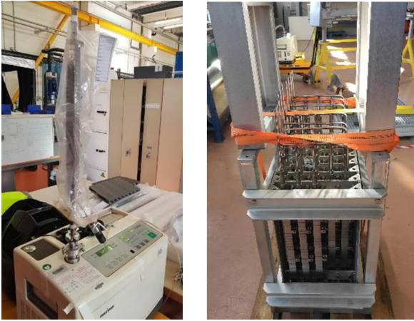
Figure 6: (Left) PFU during cold helium leak test (Right) tool enabling the hot helium leak testing of 40 PFUs in parallel
