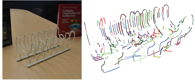
Fig. 14. For dense wire structures, assuming access to precise camera calibration and clean background, the image-based reconstruction method of Liu et al. [2017] results in many spurious 3D curves leading to significant time complexity as it requires to approximate the mTSP problem.
