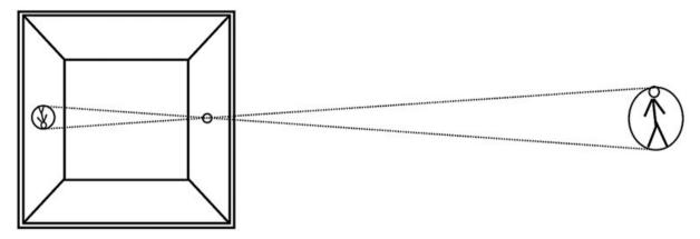
Fig. 1 Schematic view of the principles of the simplest version of a camera obscura. 6th century BC to Renaissance; China to Greece in antiquity. An image projected – by sunlight creating a shadow – from outside through a pinhole in the wall of a dark chamber appears, reversed and inversed, on the wall of the chamber opposite the pinhole.
