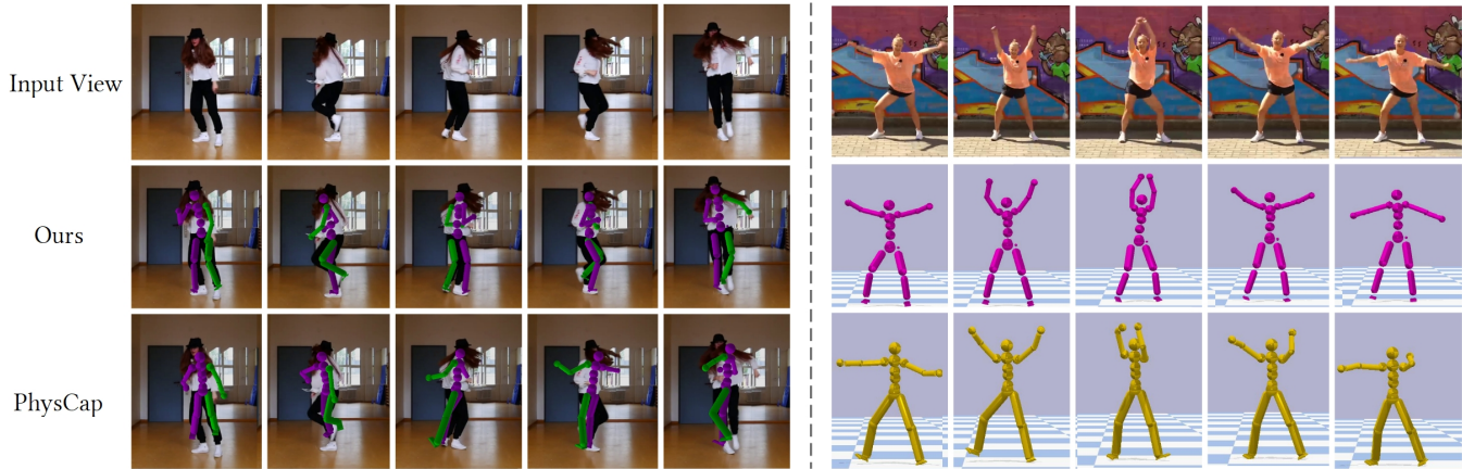
Fig. 5. Qualitative comparisons of methods with physics-based constraints on videos with fast motions. While having a consistently improved accuracy on general motions compared to PhysCap, our approach can capture significantly faster motions as it learns motion priors and the associated gains of the neural PD controller from data.
