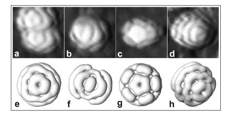
FIG. 1. Comparison of experimental STM images of individual molecules (a)–(d) with calculated shapes of C<sub>60</sub> HOMO's (e)–(h). The applied voltages and tunnel currents are 2 V, 0.2 nA (a); –1.5 V, 0.2 nA (b); 2 V, 1 nA (c); and –2 V, 1 nA (d). The theoretical images correspond to isosurfaces of constant HOMO density. Reprinted from J.I. Pascual *et al.*, Chem. Phys. Lett. **321**, 78 (2000) with permission.
