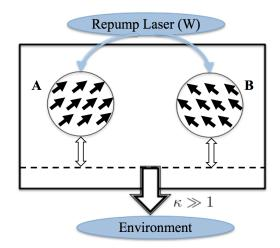
Figure 2: Cartoon depicting the driven-dissipative experimental setup with two atomic ensembles inside a bad cavity. In ensembles 'A' and 'B', the solid arrows denote individual atoms. The double-headed block arrows correspond to the Rabi coupling between the ensembles and the cavity mode (dashed line). The rate of loss of photons from the cavity is  $\kappa$ .
