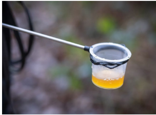
Figure 1. Urine collection device used for dogs and wolves consisting of an expandable metal stick and a plastic cup.
