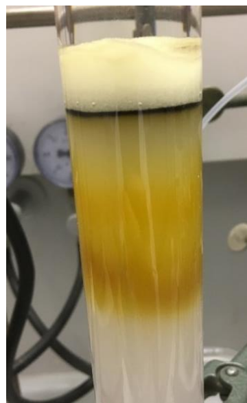
The yellow band of [BiRh(OTfa) 4 ] is eluted with toluene/MeCN (gradient 100:0 → 90:10), whereas the black impurities stick on top of the column.
