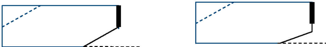
Figure 7. The figure on the left shows the 18 degree configuration. The figure on the right shows an angle of 14 degrees. Notice how the bold lined 18 degree back piece is still there, and the additional piece is added onto the original 18 degree piece in order to close gaps.
