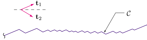
Figure 11: A wrinkled portion \mathcal{C} of the grain boundary \mathcal{S} . The angles \vartheta_1 and \vartheta_2 associated with the facet-tangents \mathbf{t}_1 and \mathbf{t}_2 must be bitangency angles of the Frank diagram.
