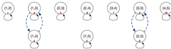
(a) Ordered state sequence S_1 consists of the 7 states in the first row, and S_2 consists of the 3 states in the second row. The states 2 and 9 are the branch and merge points of S_2 , respectively. The dashed transition links are created by Steps 2 and 3 of Algorithm 2.
