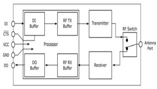
Figure9. Internal Data Flow Diagram
