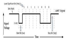
Figure8.UART data packet 0x1F transmitted through the RF module
