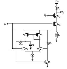
Fig.3.4 Proposed Cascode LNA with Active Inductor
