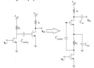
Fig.3.5 CMOS LNA with a current-reuse topology
