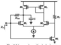
Fig. 2.2 Low noise active inductor
