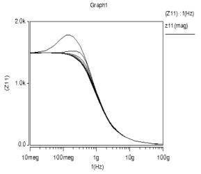
Fig4.1.Input Impedance of Active Inductor
