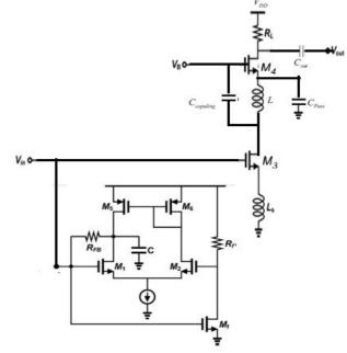
Fig.3.6 Proposed Cascode LNA with Current reuse
