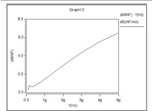
Fig.4.6 Noise figure of LNA
