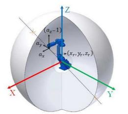
Fig. 4. The two spherical surfaces that define the robot field of operation. The "current" robot point and the acceleration vector components that will define the robot movement direction are shownin figure. Thus, in terms of robot translation movements, the pose increment is  $i = [i_1 i_2 i_3 0 0 0 i] T$
