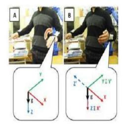
Fig. 8. Postures performed by the user left arm. A - Robot stopped. B - The robot starts the movement.
