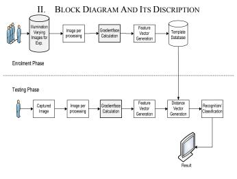
Figure.1 Block diagram of face recognition
