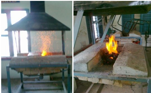
Fig 2. Forging Table for Heating
