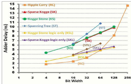
Fig. 6 . Simulation results for the adder designs
