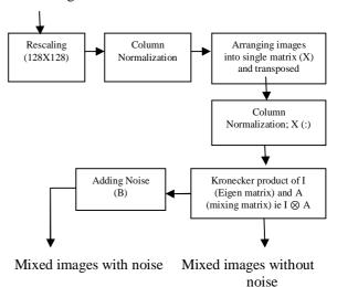
Figure 2. Mixing Process
