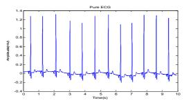
Figure 1: Input ECG signal with sampling frequency of 500 Hz
