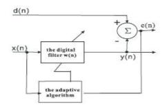
Figure 4: general Adaptive filtering diagram
