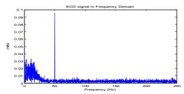
Figure 3: Noisy ECG signal (contain 50 Hz PLI and motion artifact noise) in frequency domain
