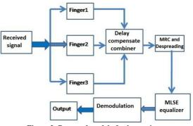
Figure 2: Proposed model of rake receiver.
