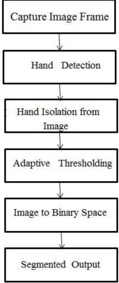
Figure 3: Flow Chart for Proposed model
