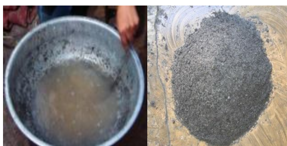
Fig2: Binder preparation and carbonized charcoal mixed with the binder
