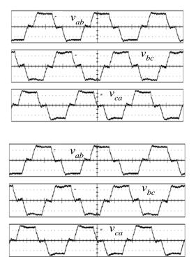
Fig. 6 : Waveforms of Three-phase voltage source inverter (a) output phase voltages and phase currents (b) Output line voltages Scales: time  $1\mu$ S/div., voltage 100 V/div., current 10 A/div.
