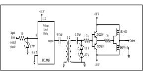
Fig. 5 : Bipolar Gate driver circuit
