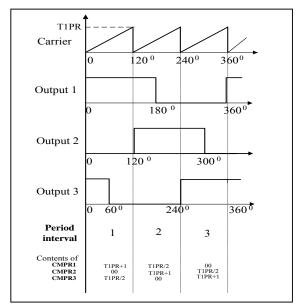
Fig.4 : Generation of PWM gating signals for three-phase inverter.
