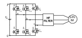
Fig. 1 : Three-phase Voltage Source Inverter feeding three-phase Induction Motor.
