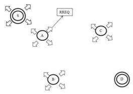
Fig. 1: Broadcast of Route Request Packet
