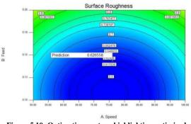
Figure 5.10- Optimation contour highlighting optimized (lowest) value of surface roughness at a Particular setting.
