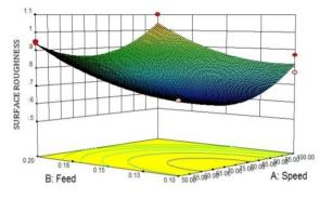
Figure 5.6 - Surface roughness 3D surface in cutting speed and feed rate plane at depth of cut of 0.150mm
