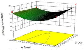
Figure 5.9 - Surface roughness 3D surface in cutting speed and depth of cut plane at feed of 0.02 mm/rev
