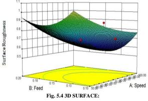
Figure 5.4 - Surface roughness 3D surface in cutting speed and feed rate plane at depth of cut of 0.1mm
