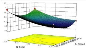
Figure 5.5 - Surface roughness 3D surface in cutting speed and feed rate plane at depth of cut of 0.125mm
