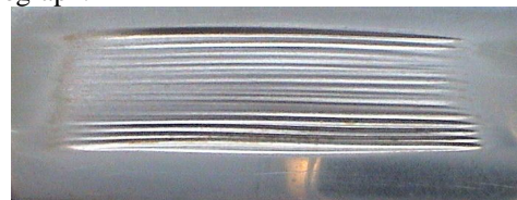
Fig. 8 (a) : Photograph of worn out surface of mild steel after slurry abrasion test with 300-450 µm silica sand particles at load of 125 N.
