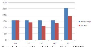
Figure 6: Average end-to-end delay in multichannel WMN.
