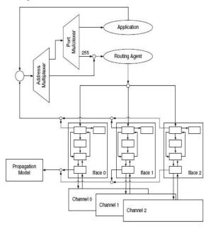
Figure 2: Mobile Node Architecture with Multi-channel support
