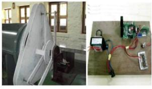
Fig.4.Variable frequency Drive for speed control
