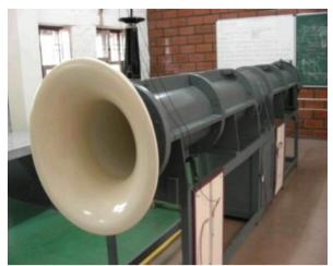
Fig: 2 Ducted Axial Fan Rig
