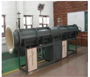
Fig: 3 Side View of Ducted Axial Fan Rig
