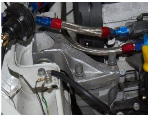
Fig. 5 : Mounted engine bracket.
