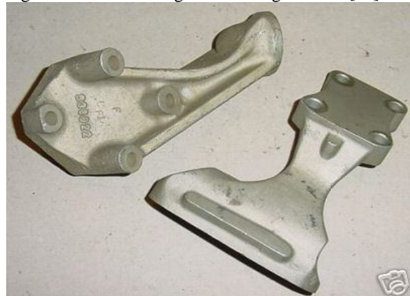
Fig. 2 : Aeroplane engine's continental engine mounting Bracket
