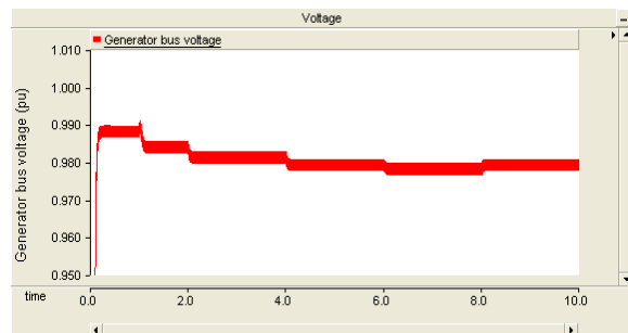
Fig-2: Variation in generator bus voltage due to step change in load (with no reactive power support)
