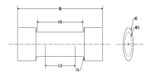
Fig.3. Tensile Test Specimen Geometry.
