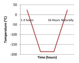
Fig.2. Cryogenic Process steps involved.
