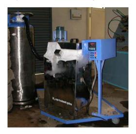
Fig.1. The Cryogenic Treatment Chamber
