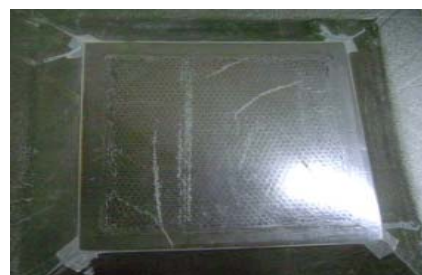
Fig.10.stabilize core with PU solid foam
