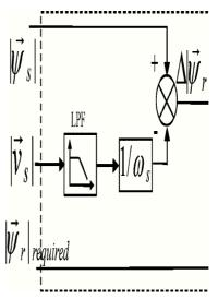
Fig .3 Rotor flux reference generation strategy
