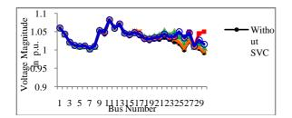
Fig. 4: Voltage profile of IEEE 30 Bus system for normal loading condition
