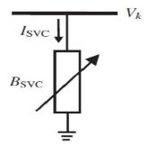
.Fig. 1: Variable shunt susceptance model The current drawn by the SVC is given in (14).  $I_{SVC} = iB_{SVC}V_k(14)$
