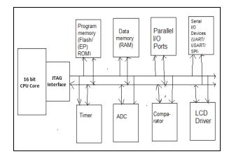
Fig. Block diagram of MSP 430 uC
