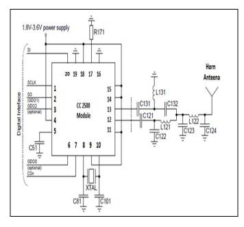
Fig2. Pin diagram of CC2500 module.
