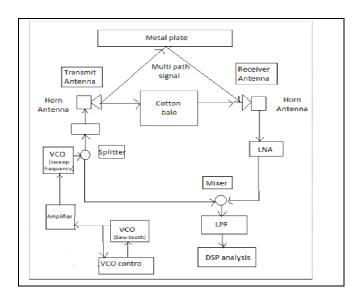
Fig.1 Schematic layout of detection of moisture
