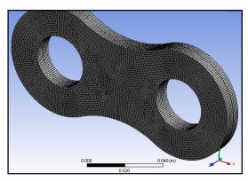
Fig. 8: Shows the meshed model with 1mm element size
