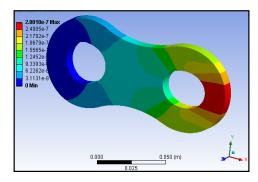
Fig. 10: Deformation in link
