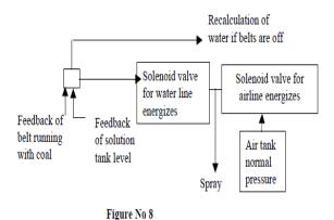
The solenoid valves (airline and waterline) of headers are energized if conveyor is running with coal. If all or some of the solenoid valves for water line are not energized the system will realize pressure through pressure relief valve, which protects the system. A solenoid valve for water line is provided with bypass line, which operates when none of the spray header
