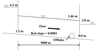
Figure 5. Schematic diagram of the single-pool canal used for testing the canal automation software.
