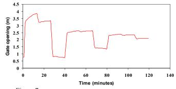
Figure 7. Variation of the upstream gate opening of the single-pool canal with time during control
