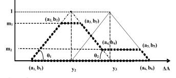
**Figure 4.** Computing the output membership function by implication. The values of  $a_2$ ,  $a_3$ ,  $a_4$  and  $a_5$  shall be obtained as follows: **Calculation of a**<sub>2</sub>
