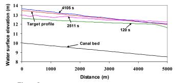
Figure 8. Development of water surface profiles with time in the single-pool canal during control
