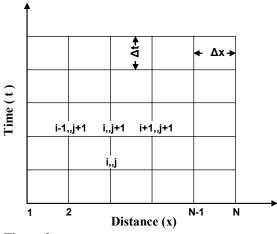
**Figure 2.** Computational domain for the fuzzy control algorithm: N = number of nodes in the x – direction, i = node number in the x – direction, j = node number in the t – direction.
