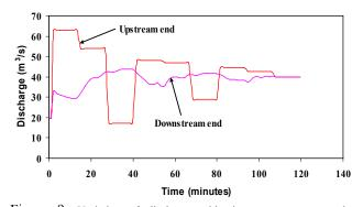
Figure 9. Variation of discharge with time, at upstream and downstream ends of the single-pool canal during control
