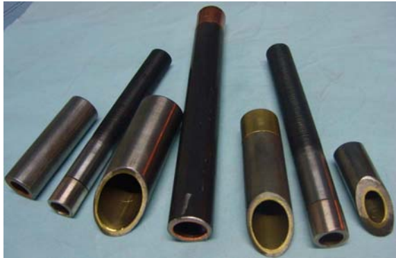
Fig. 2. Some types of bi-layered tubes [2]
