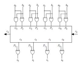
$\begin{array}{l} C_4 = G_3 \, + \, P_3 \; G_2 \; + \! P_3 \; P_2 \; G_1 \; + \! P_3 \; P_2 \; P_1 \; G_0 \, + \; P_3 \; P_2 \; P_1 \\ P_0 \; C_0 \end{array}$
