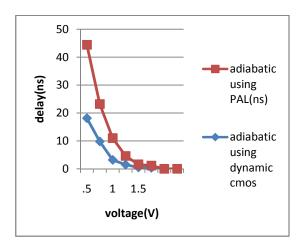
From the graph we see that power consumption and delay both decrease when supply voltage is increase in the adiabatic CLA using dynamic CMOS logic while in the adiabatic CLA using PAL power consumption decrease but delay is increase. So from the simulation result it is clear that adiabatic circuit using dynamic CMOS logic has higher speed and lower power consumption.
