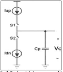
Fig. 1. Single ended charge pump model
