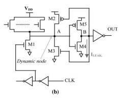
Figure 3. Previous works showing OR gate a. Diode footed Domino [6] b. Domino circuit in scheme [7]
