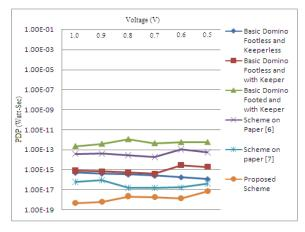
Figure 7. PDP Plot for the proposed scheme with the other schemes by reducing  $V_{\text{DS}}$  from 1 V to 0.5 Mv
