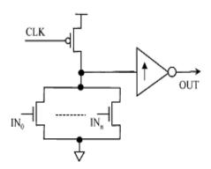
Figure 1. A typical footless Domino OR gate
