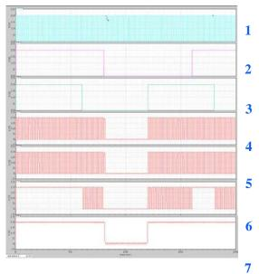
Figure 6. Waveform simulated for the OR gate
