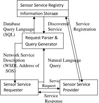
Figure 3: Proposed Architecture for Sensor Service Discovery(x-SOA)
