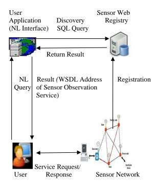
Figure 5: Operation of the prototype system
